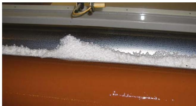
now be turned off. To guarantee a seal the nozzle can be coated with KLEIBERIT 761.7/9 cleaner (block format). This coat must be removed before the next process is started.
