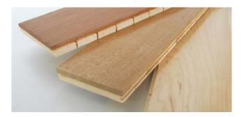
In 3-layer parquet production, three layers are glued together to form a composite. However, since essentially flat materials are bonded together, adhesives should preferably be applied as a film. PVAc dispersions or EPI systems are frequently used. However, modern system concepts rely on PUR hotmelts and their advantages.
