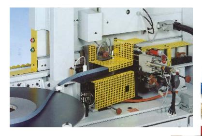
The operating temperatures for PUR Hotmelt lie, depending on the PUR type, between 120°C and 160°C (248°F and 320°F). Because PUR Hotmelts react with air moisture, the application device should be cleaned after use or stored in a nitrogen pressure tank.
