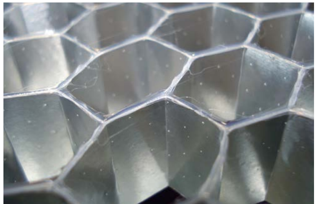
Aluminium honeycomb bonded with aluminium cover layers with KLEIBERIT 543.8 2C PUR adhesive.
