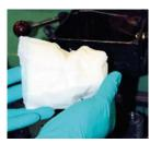
Step 4: Place the adhesive block in the pre-heated melting tank.
