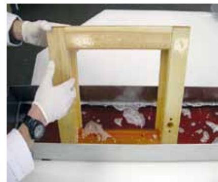
Immerse manufactured window frames in a basin
