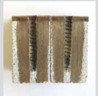
Cross section: KLEIBERIT 555.6 strengthened drill hole in mineral board. Clearly visible the inner thread created by the screw.
