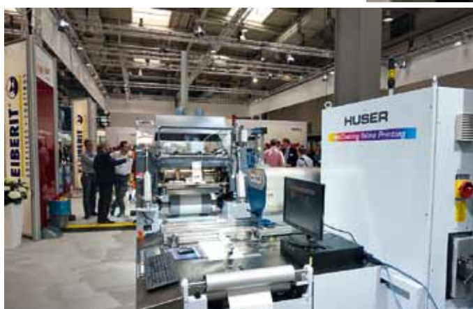
400 mm inline digital printing line in Hanover, for printing and subsequent "HotCoating" in one pass.
