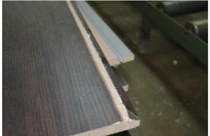
An example of where the cutters chipped away the edging that delaminated during profiling
