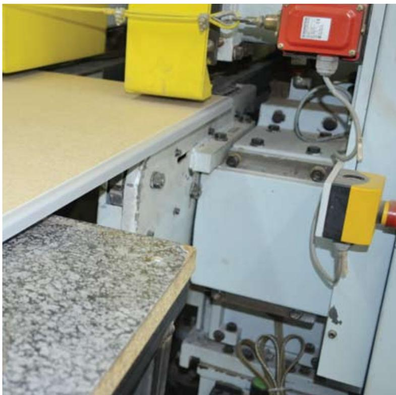
A board with a sofformed profiles edge coming off the Homag line. Here the melamine paper edging can be seen properly applied using Kleiberit 735.0
