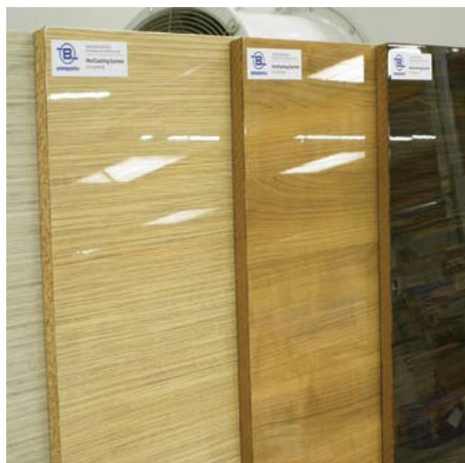
High gloss boards produced using Kleiberit's HotCoating technology
