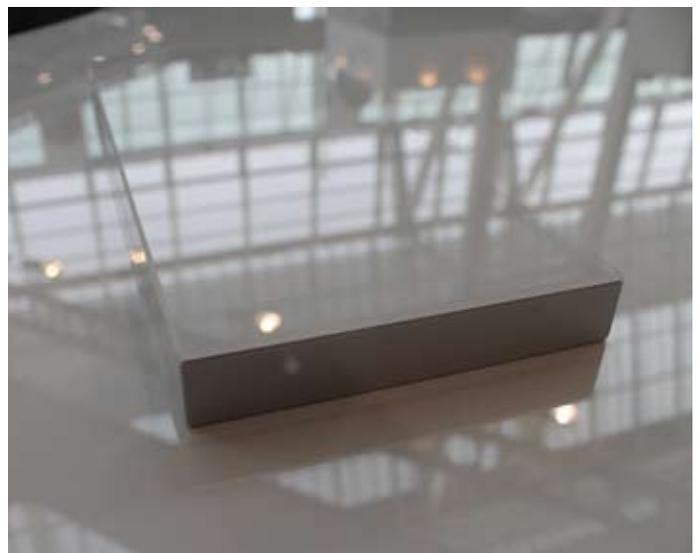
Kleiberit HotCoating can be used to upgrade standard chipboard panels into a white super high gloss finish
