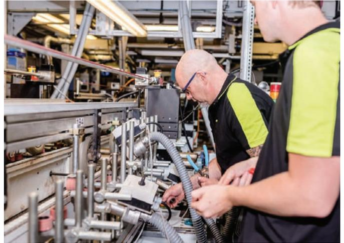
With foil wrapping the company's core competence for decades, Spaljisten today has several wrapping lines installed and is thus able to offer profiles with 2D and 360 degree wrapping technology. One of the lines is unique as it is specialised in processing thicker foils that mainly have a high gloss finish that is used for fronts and panels; these panels fulfil the highest requirements when it comes to top quality surfaces.
