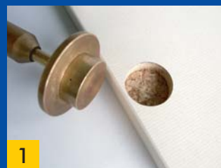
1 glue is pressed through small holes into hinge recess
