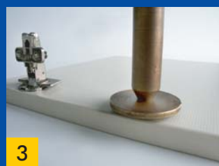
3 Applicator cylinder in bottom position while pressing 555.6 glue into hinge recess
